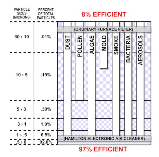
ALL FILTERS, WHETHER THEY ARE STANDARD FILTERS OR ELECTRONIC AIR FILTERS, STATE THEIR EFFICIENCY REATINGS. THOUGH SOME CLAIM TO BE ABOVE 90% EFFICIENT, THEY DO NOT STATE TO WHAT DEGREE OR SIZE MICRON PARTICLE THEY ARE RELATING TO. THERE ARE MANY FILTERS STATING SUCH HIGH EFFICIENCY RATINGS BUT LIMIT THEIR CLAIM TO SUCH PARTICLES THE SIZE OF 5 MICRONS OR LARGER.
