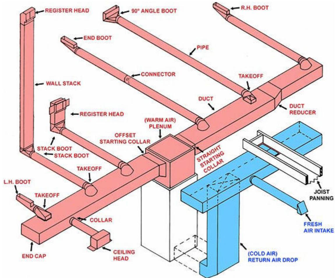
The size of each component is determined by the airflow that needs to pass through it. The overall sizing of the "Trunk Line" is designed to evenly distribute the appropriate amounts of air to every register. Caution must always be used when sizing individual components to insure that the heating/cooling equipment has adequate airflow for optimum performance.
