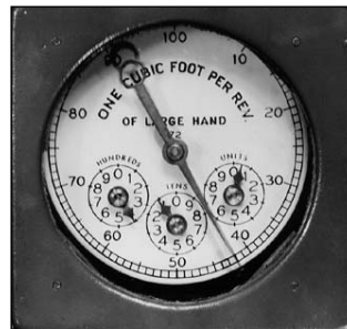
Figure 12.1 Dials of Typical Gas Meter
