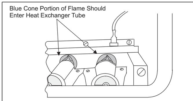
**FIGURE 5:** Burner Flame Drawing (Upflow Configuration Shown)
