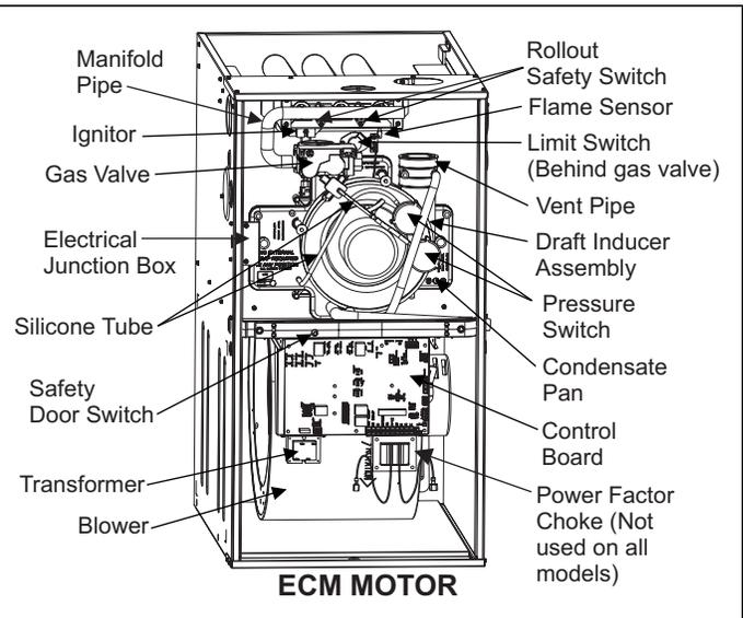
FIGURE 4: Component Location - 97% Modulating ECM Models
