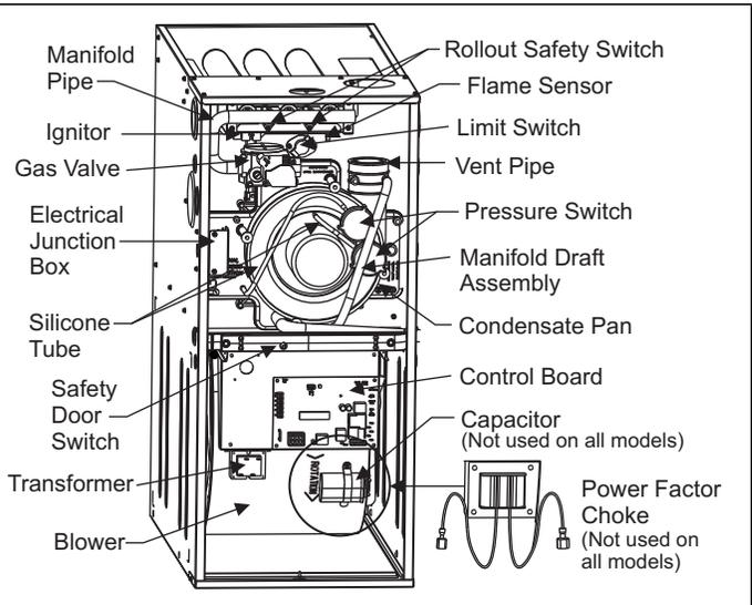
FIGURE 2: Component Location - 95% Single & 96% Two Stage Models
