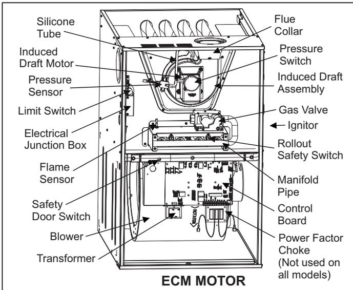
FIGURE 3: Component Location - 80% Modulating ECM Models
